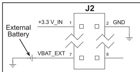
**Figure C-1. External Battery Connections at Header J2**
