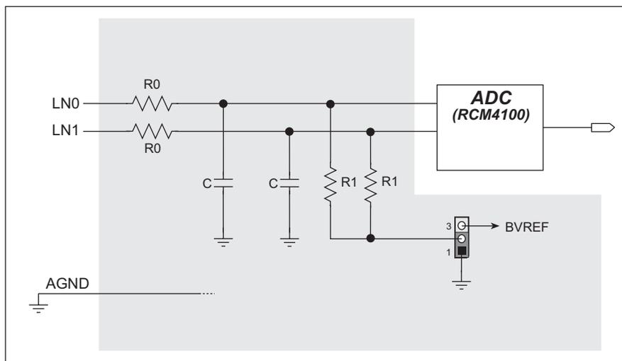
**Figure 9. Resistor Divider Network for Analog Inputs**
