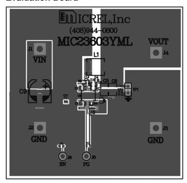
Figure 1. MIC23603 Evaluation Board - Top Layer
