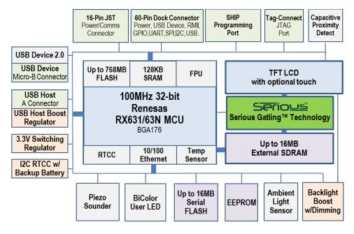
SIM231 Hardware Block Diagram options depend on variant selected
