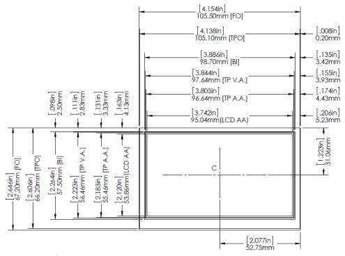
These two diagrams are critical for correct bezel design. The acronyms in the above LCD diagram are as follows:
