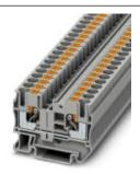
Feed-through terminal block, Connection method: Push-in connection, Cross section: 0.5 mm<sup>2</sup> - 10 mm<sup>2</sup>, AWG: 20 - 8, Width: 8.2 mm, Height: 42.2 mm, Color: red, Mounting type: NS 35/7,5, NS 35/15
