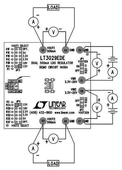
Figure 1. Proper Measurement Equipment Setup
