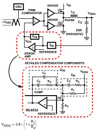
FIGURE 5. VOLTAGE-MODE BUCK CONVERTER
