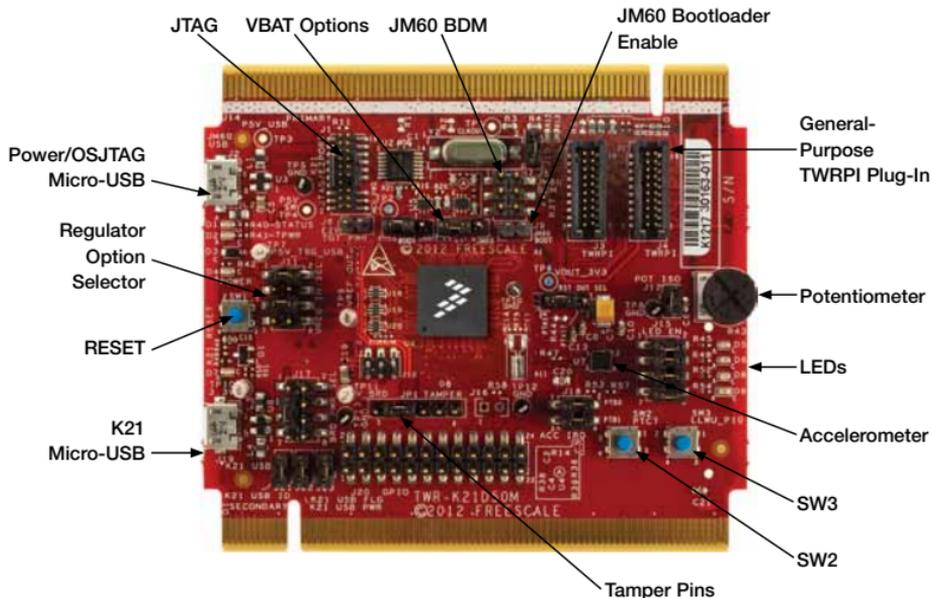
**Figure 1:** Front side of TWR-K21D50M module (TWRPI devices not shown).
