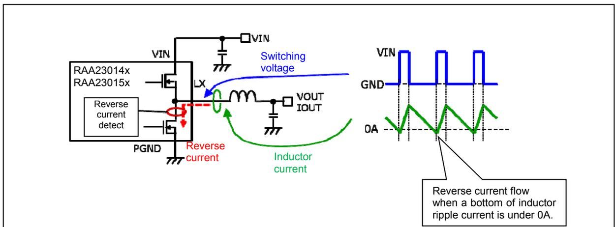
RAA23014x has x\_autoPFM pin. When Low level, the devices operate Auto PFM mode (PFM mode / PWM mode changed automatically). When High level, the devices operate PWM mode, then not change into Auto PFM mode.
