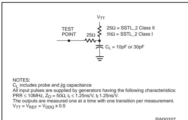
**Figure 1. Load circuitry**
