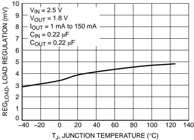
Figure 11. Load Regulation vs. Temperature
