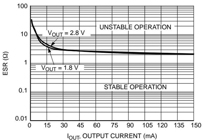
Figure 31. Output Capacitor ESR vs. Output Current
