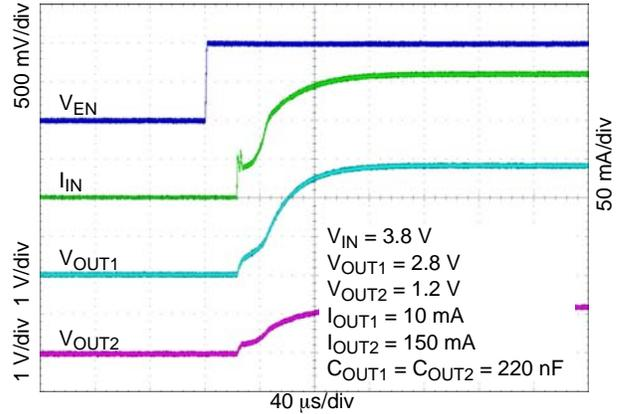
Figure 35. Enable Turn-on Response - VR1 = 10 mA, VR2 = 150 mA
