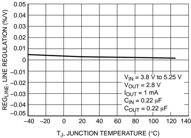
Figure 9. Line Regulation vs. Temperature
