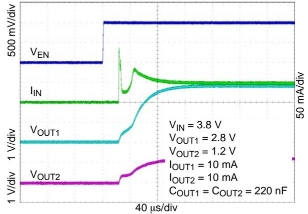
Figure 33. Enable Turn-on Response - VR1 = 10 mA, VR2 = 10 mA
