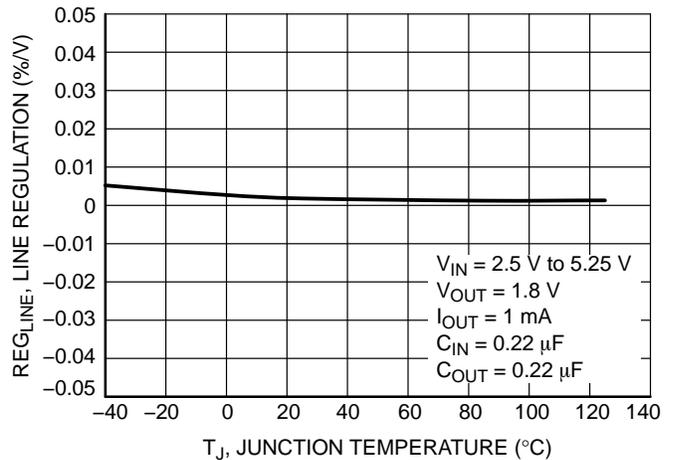
Figure 8. Line Regulation vs. Temperature
