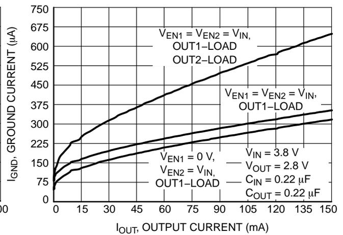
Figure 6. Ground Current vs. Output Current –
