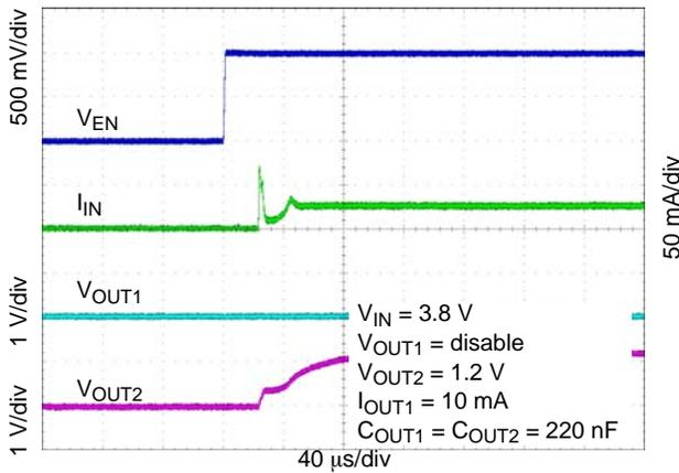
Figure 32. Enable Turn-on Response - VR1 = Off, VR2 = 10 mA
