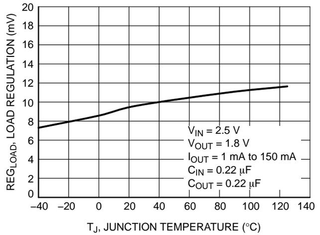
Figure 10. Load Regulation vs. Temperature
