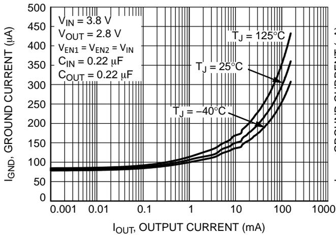
Figure 5. Ground Current vs. Output Current –
