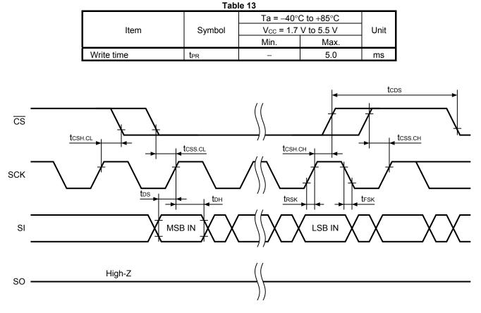
Figure 4 Serial Input Timing
