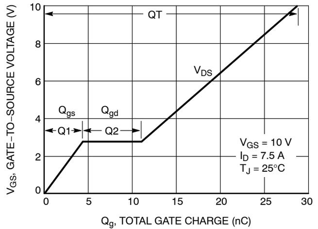
Figure 8. Gate-to-Source and Drain-to-Source Voltage vs. Total Charge
