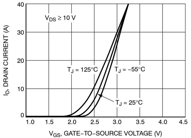
Figure 2. Transfer Characteristics
