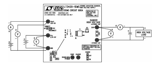
Figure 1. Proper Measurement Equipment Setup
