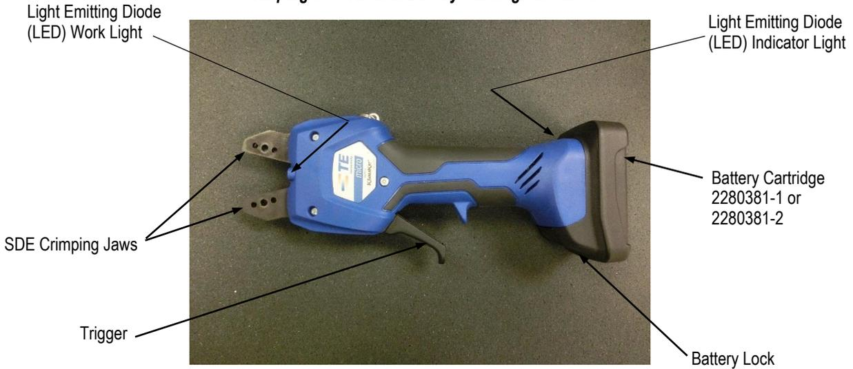
**CRIMPING TOOL (With Battery Installed)**
