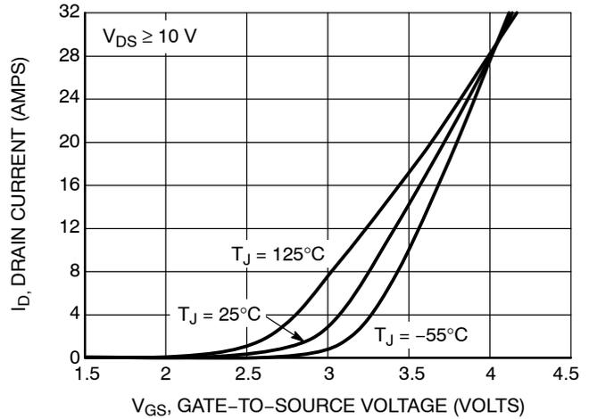
**Figure 2. Transfer Characteristics**
