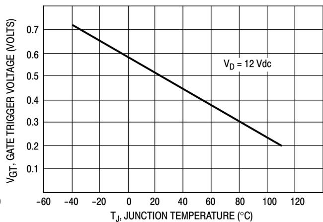
Figure 4. Gate Voltage
