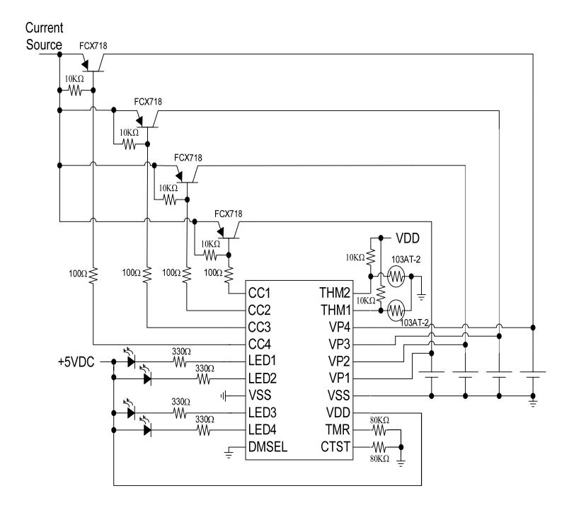
Figure 3. Application Example: Regulated Current Source Charger
