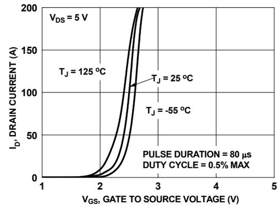
Figure 5. Transfer Characteristics
