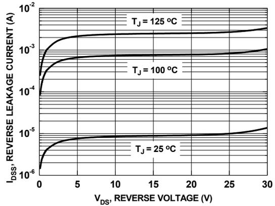
Figure 15. SyncFET<sup>™</sup> Body Diode Reverse Leakage vs. Drain-Source Voltage
