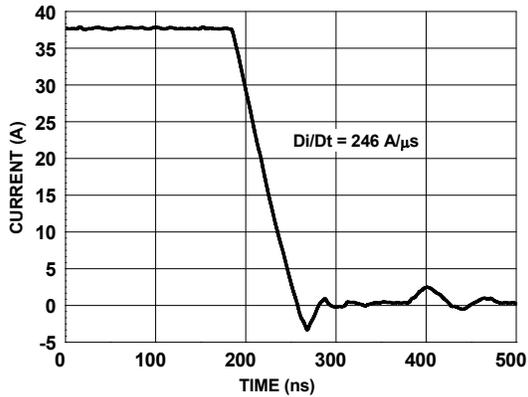
Figure 14. FDMS1D4N03S SyncFET<sup>™</sup> Body Diode Reverse Recovery Characteristic
