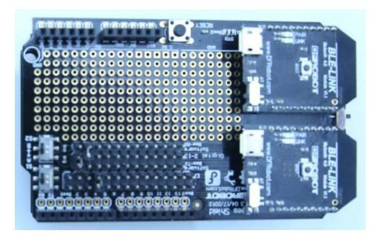
Bee1 <==> Hardware Serial Port; Bee2 <==> Software Serial Port
