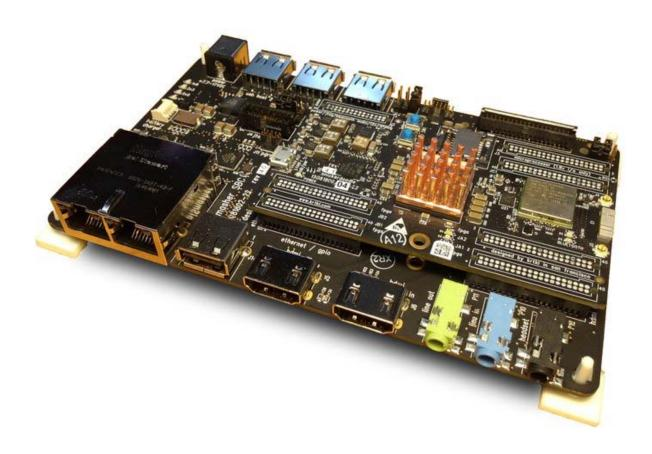
Or maybe what you're looking for is gigabit Ethernet, high-speed USB, a bunch of reconfigurable I/O, and...simultaneous HDMI output AND input? Enter: piSmasher... Named "piSmasher" for a reason, you'll get everything Raspberry Pi provides and more - you can kind of think of it as a Raspberry Pi on steroids.
