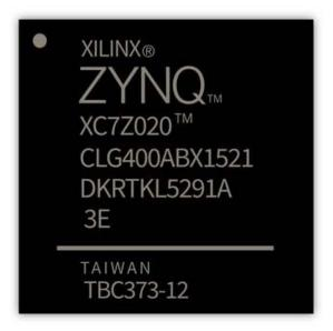
Unlike a lot of more complicated reconfigurable hardware, the Zynq SoC inside snickerdoodle has a full-blown ARM microprocessor inside meaning you are able to treat it (and program it) as if it were "just another microprocessor"...with a ton of really fast, reconfigurable I/O.
