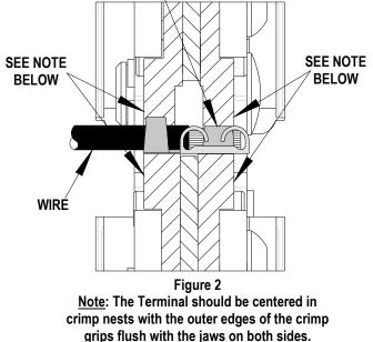
2. Before attempting to crimp any terminals, make sure all the upper tooling is correctly placed into the upper jaw. The desired nest being used for the proper wire size should be in the forward position, (The marking on the upper tooling "A" for 1.0mm<sup>2</sup> or "B" for 18 AWG and 0.8mm<sup>2</sup>). This is done by removing the knurled fastener that holds the upper tooling in place and then rotating it 180° to the correct position. Then, re-installing the fastener. See Figure 1.
