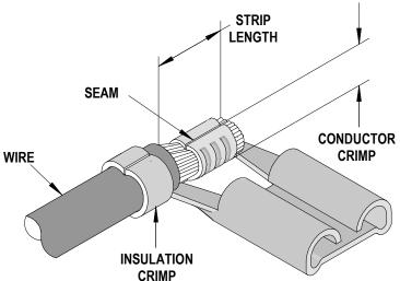
The above terminal drawing is a generic terminal representation. It is not an image of any terminal listed in the scope.
