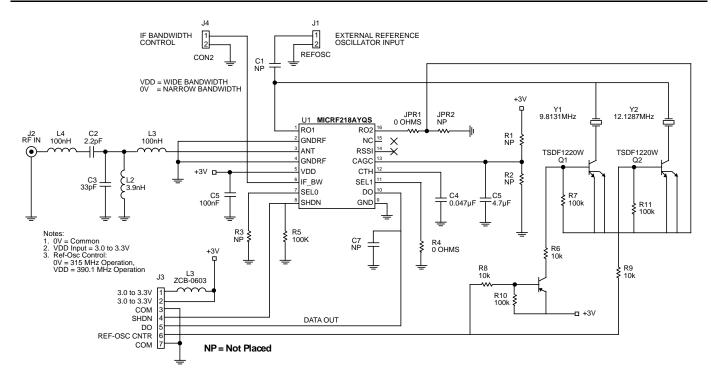
Figure 4. Dual Frequency QR218BP\_SWREF, 315 MHz and 390 MHz
