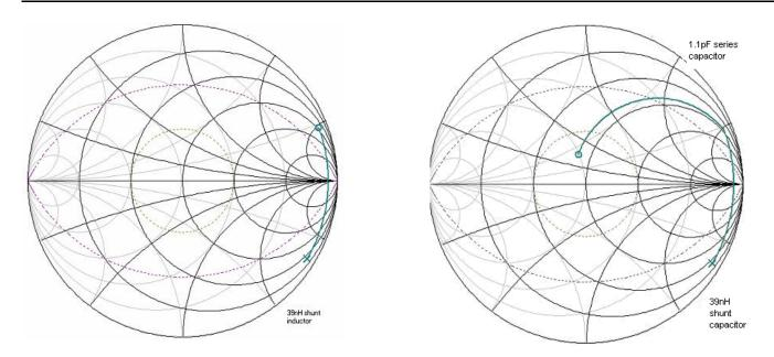
Figure 9. Plotting the Shunt Inductor and Series Capacitor
