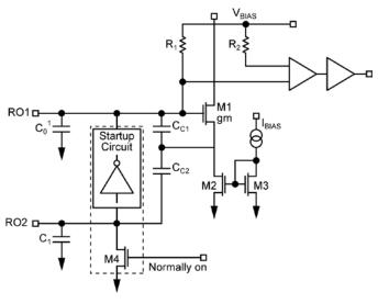
Figure 6. Reference Oscillator Circuit
