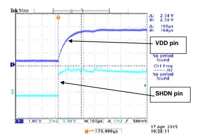
The suggestion provided above will generally serve to prevent the startup issue from happening to the MICRF218 series ASK receiver. However, exact values of the RC network depend on the ramp rate of the supply voltage, and should be determined on a case-by-case basis.
