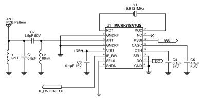
315MHz/315.802, 900Hz Baud Rate Example
