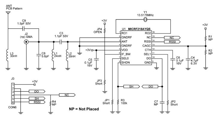
Figure 7. QR218HE1 Application Example, 433.92 MHz, Narrow Band
