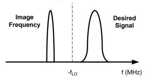
Figure 10. Low Side Injection Local Oscillator
