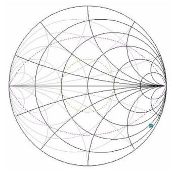
Figure 8. Device's Input Impedance, Z = 9.54-j152 $\Omega$
