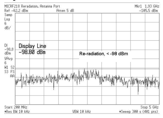
Re-radiation from MICRF218 Antenna Port
