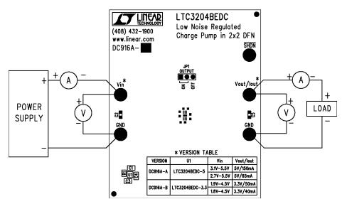
Figure 1. Proper Measurement Equipment Setup
