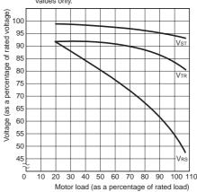
Note: For phase loss of phase R.  $V_{ST}$ ,  $V_{TR}$ , and  $V_{RS}$  indicate the motor terminal voltage at phase loss.
