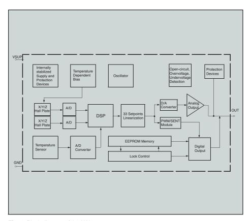
Fig. 1: Block diagram of the HAL 37xy
