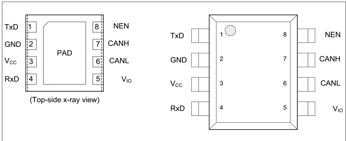
Figure 2 Pin configuration
