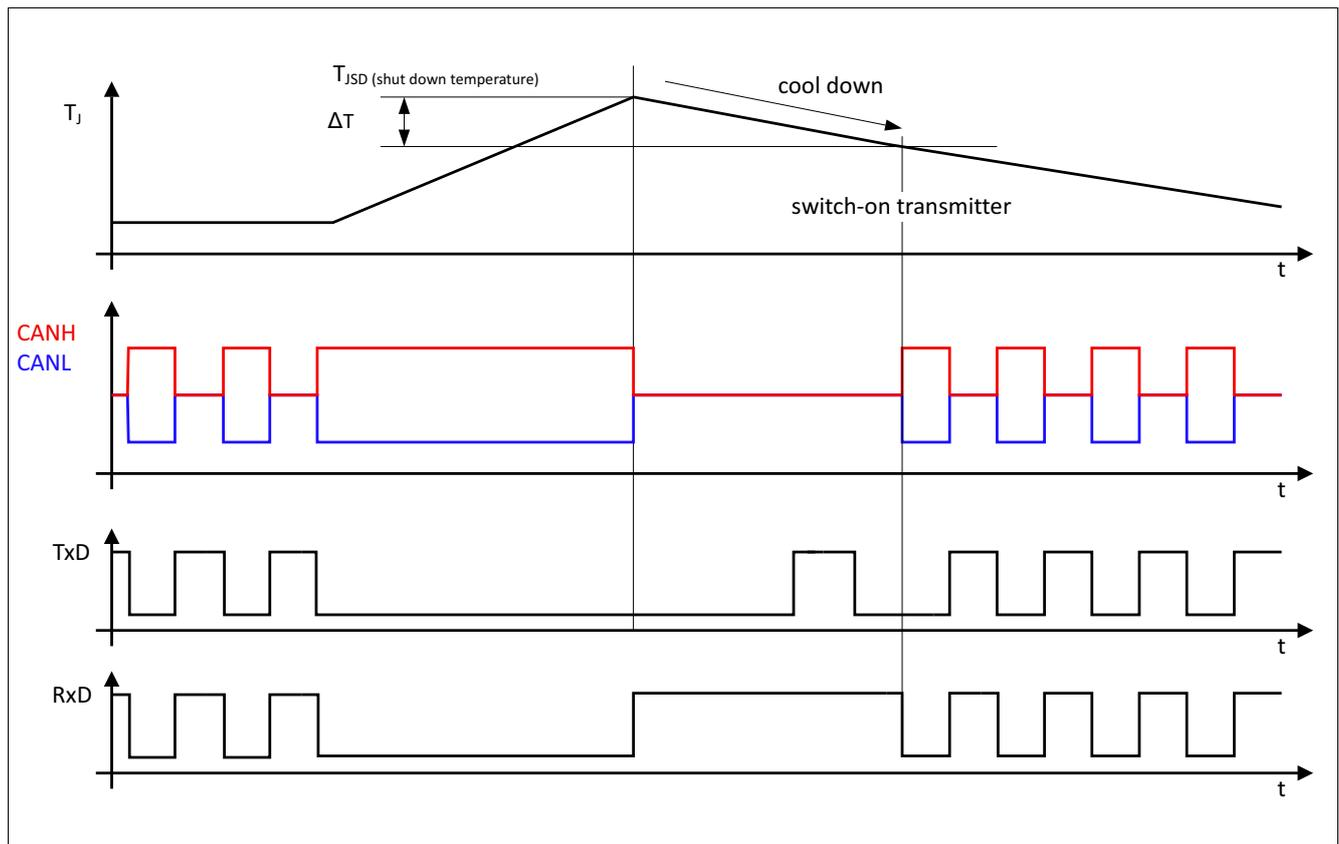
Figure 9 Overtemperature protection
