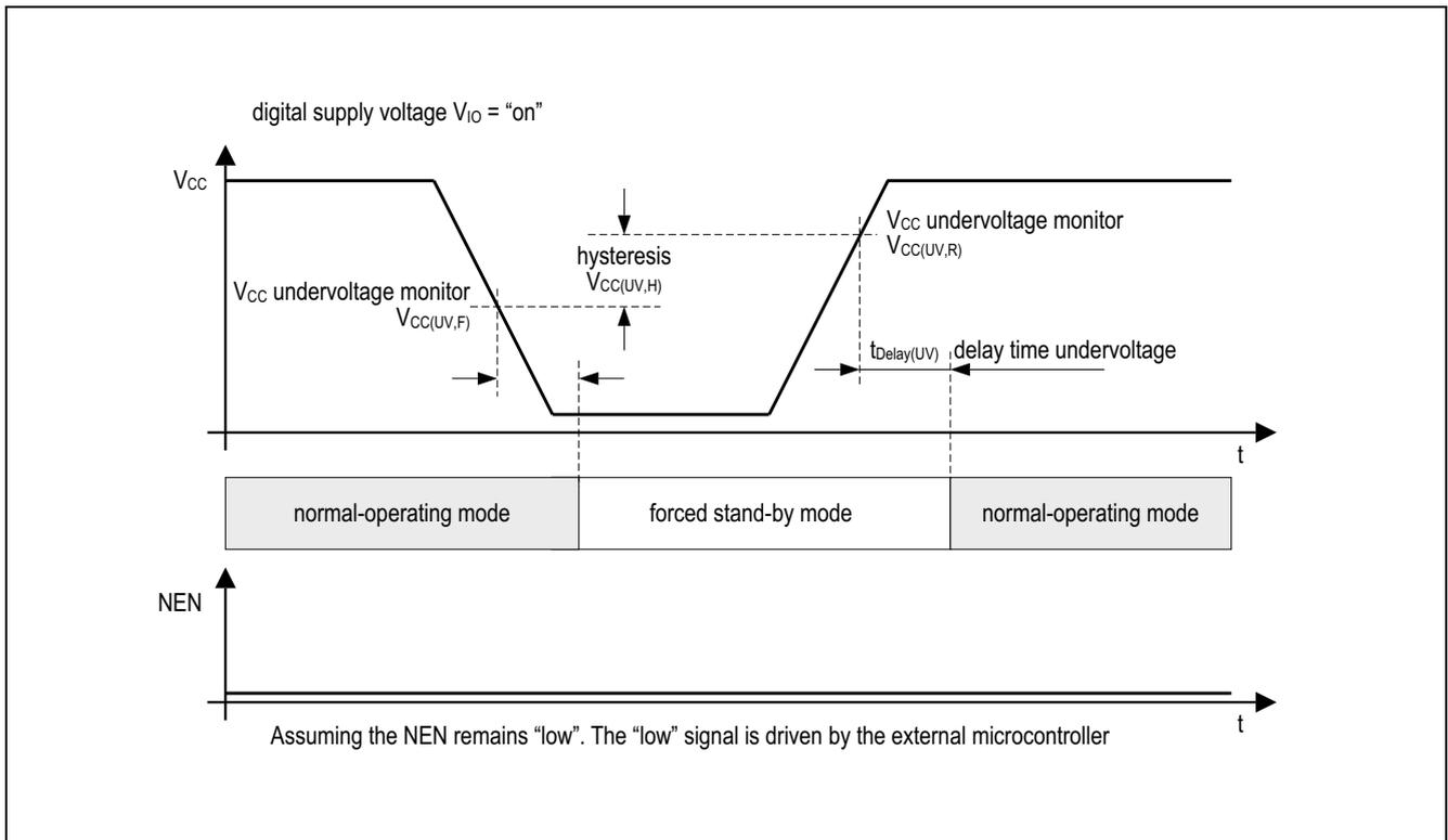
Figure 7 Undervoltage on the transmitter supply  $V_{CC}$
