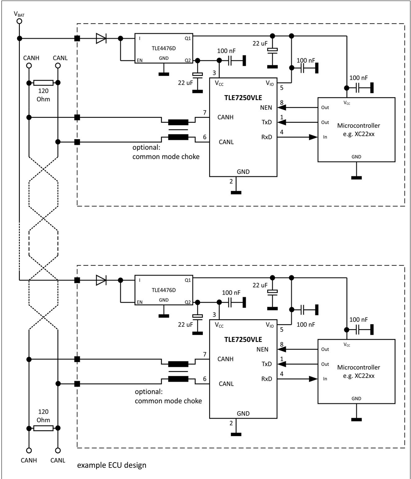
Figure 13 Application circuit
