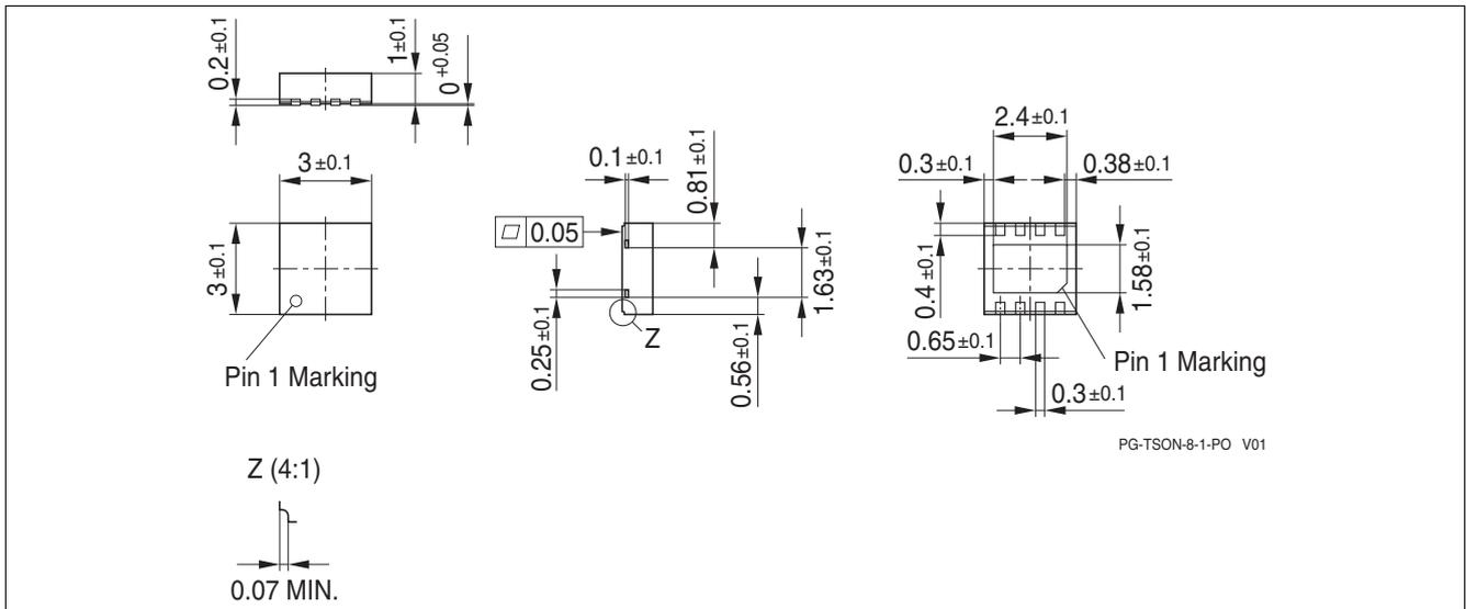
Figure 16 PG-TSON-8 (Plastic Thin Small Outline Nonleaded PG-TSON-8-1)
