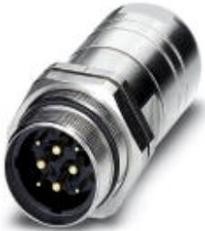
Rear panel feed-through, straight, Screw locking, M40, Number of positions: 2+3+PE, Type of contact: Male connector, Crimp connection, Axial O-ring, Central fixing, Shielded: Yes, Cable cross section: 9 mm...12.5 mm
