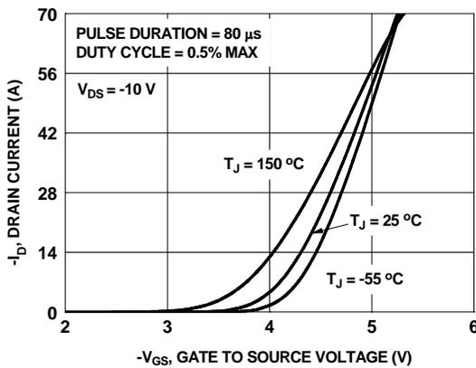
**Figure 5. Transfer Characteristics**
