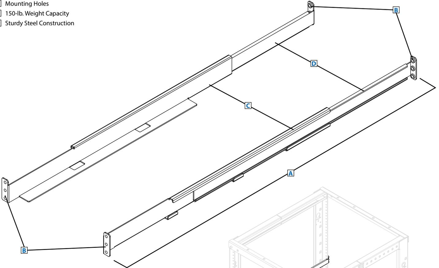
The 4POSTRAILKIT1U is an adjustable rackmount shelving system that supports 1U UPS systems as well as other 1U networking or power protection equipment. Expandable mounting rails offer front-to-rear support for equipment with 17.5-inch wide rectangular chassis and adjust to any setting between 20.5 and 36 inches. The 4POSTRAILKIT1U includes mounting hardware compatible with square-hole racks and supports weights of up to 150 lb.
