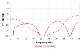
Typical IC performance measured on-wafer
