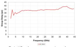
Typical IC performance measured on-wafer
