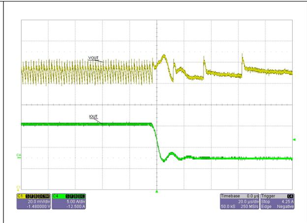
Figure 29. Over-voltage protection, VOUT = 1.5 V
