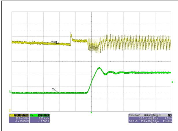
Figure 28. 5 A to 0 A VOUT load transient, Pulse-Skip
