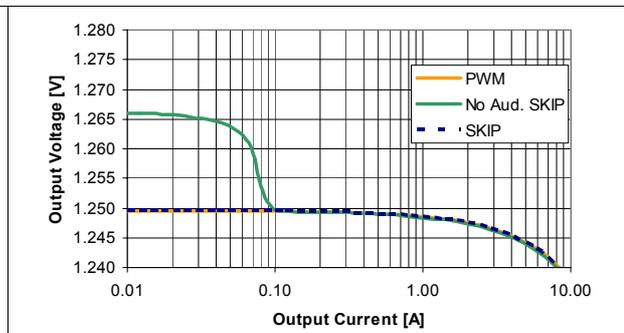
**Figure 7. VOUT load regulation, 2.5 V, Vin = 12 V**
