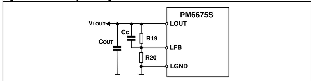
A compensation capacitor  $C_c$  must be added to adjust the dynamic response of the loop. The value of  $C_c$  is calculated according to the desired bandwidth of the LDO regulator and depends on the value of the feedback resistors. In most of applications the pole due to the compensation capacitor is placed at 100-200 kHz (equation 24).
