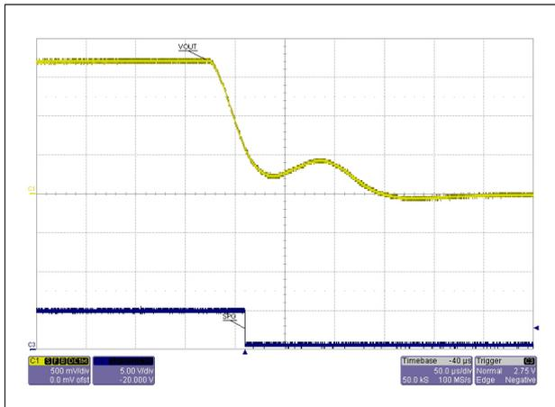
Figure 30. Under-voltage protection, VOUT = 1.5 V
