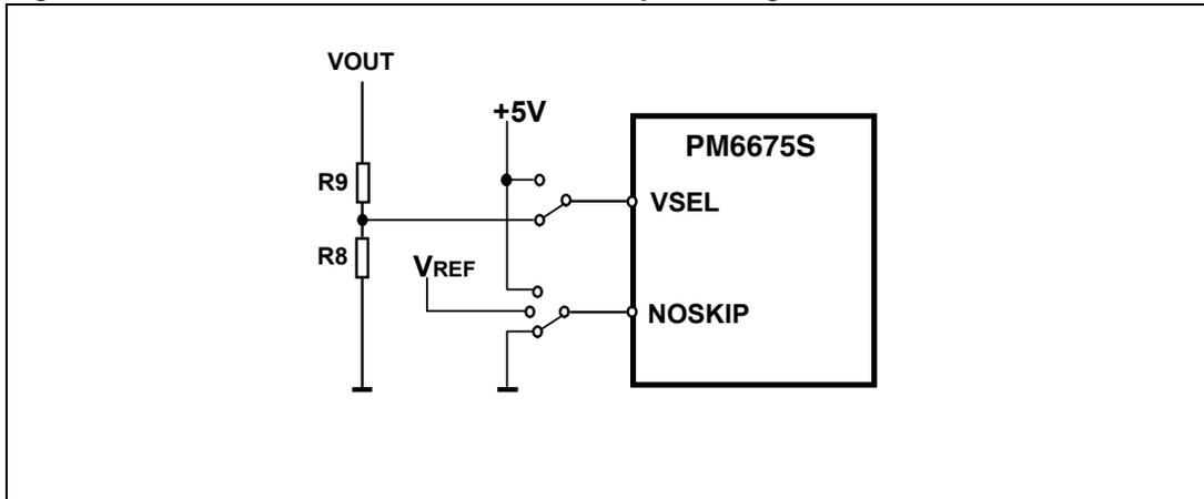
The PM6675S has been designed to satisfy the widest range of applications. The device is provided with some multilevel pins which allow the user to choose the appropriate configuration. The VSEL pin is used to firstly decide between fixed preset or adjustable (user defined) output voltages.
