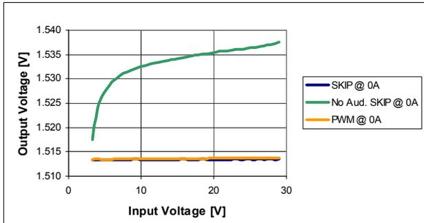
Figure 10. VOUT line regulation, 1.25 V, 0 A
