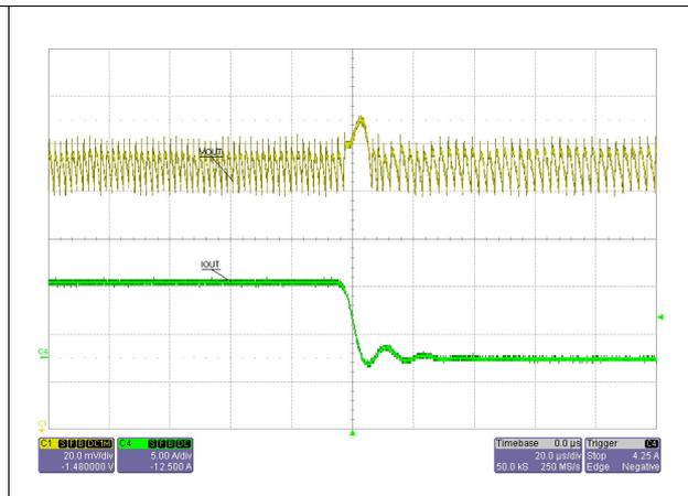
Figure 27. 0 A to 5 A VOUT load transient, Pulse-Skip
