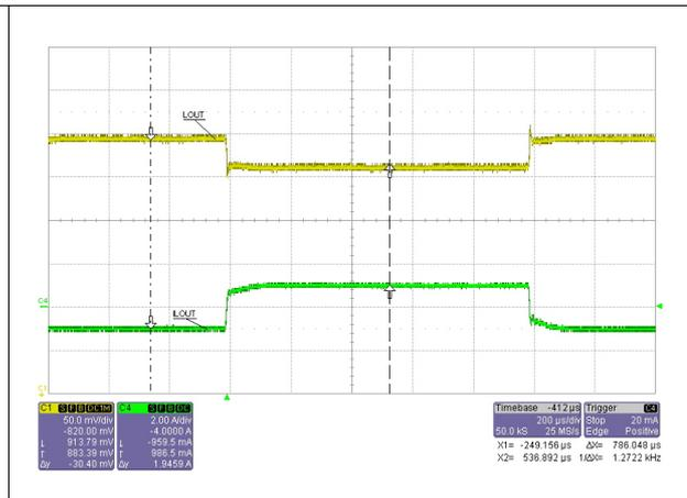
Figure 25. 0 A to 8 A VOUT load transient, PWM
