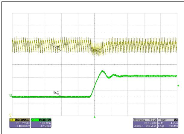
Figure 26. 8 A to 0 A VOUT load transient, PWM
