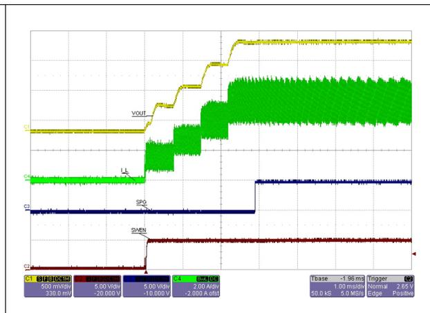
Figure 21. Switching section output soft-end
