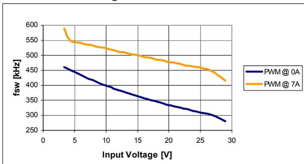
Figure 14. Switching frequency vs input voltage, 1.25 V
