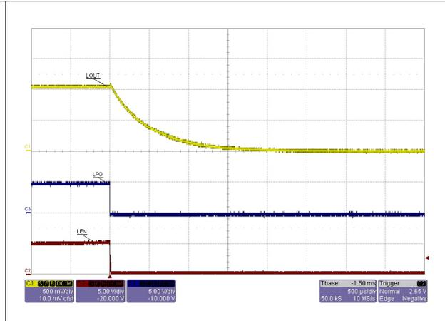
Figure 23. -1.8 A to 1.8 A LOUT load transient, 0.9 V
