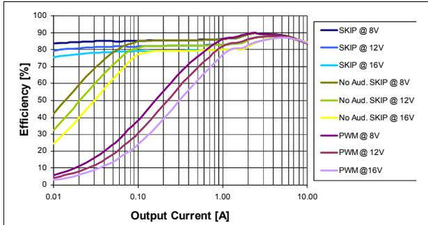
**Figure 4. VOUT efficiency vs load, 1.25 V, SW frequency = 400 kHz**
