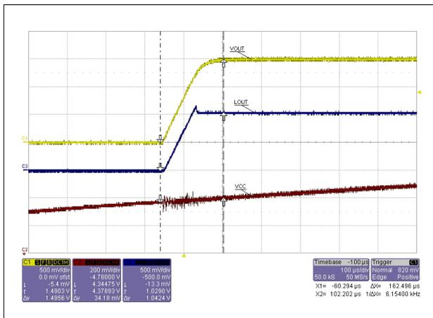
Figure 20. VOUT soft-start, 1.5 V, heavy load
