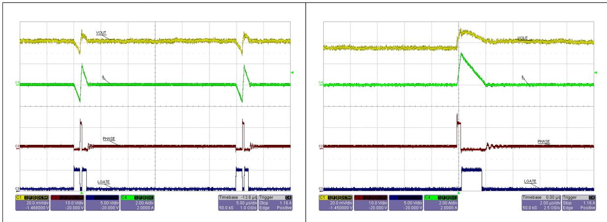
Figure 19. Power-up sequence VCC above UVLO
