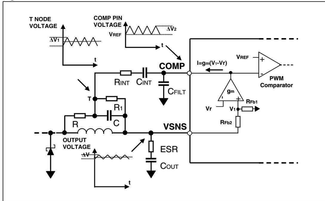
The ripple on the COMP pin is the sum of the output voltage ripple and the triangular ripple generated by the Virtual-ESR Network. In fact the Virtual-ESR Network behaves like another equivalent series resistor  $R_{VESR}$ .
