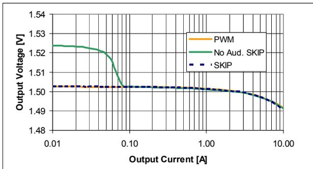
**Figure 6. VOUT load regulation, 1.25 V, Vin = 12 V**
