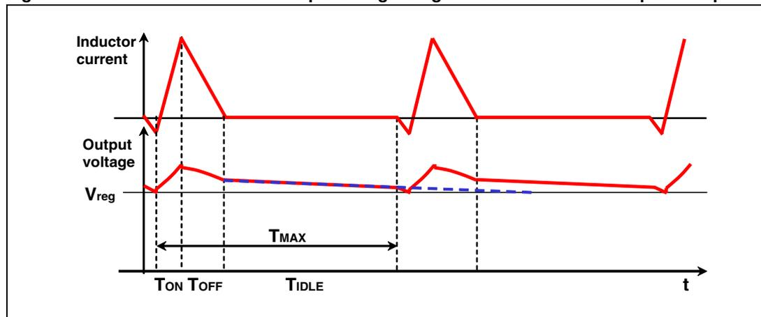
For frequencies higher than 33 kHz (due to heavier loads) the device works in the same way as in Pulse-Skip mode. It is important to notice that in both Pulse-Skip and No-Audible Pulse-Skip modes, the switching frequency changes not only with the load but also with the input voltage.
