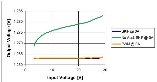
Figure 11. VOUT line regulation, 1.5 V
