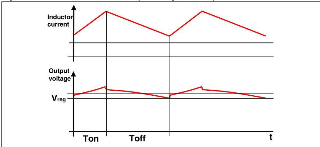
The duty-cycle of the buck converter is, in steady-state conditions, given by
