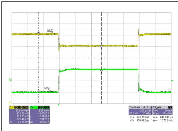
Figure 24. -1 A to 1 A LOUT load transient, 0.9 V
