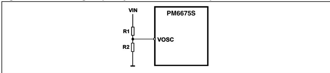
The voltage seen at this pin must be greater than 0.8 V and lower than 2 V in order to ensure the system linearity.
