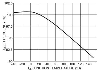
Figure 4. Oscillator Frequency Versus Junction Temperature
