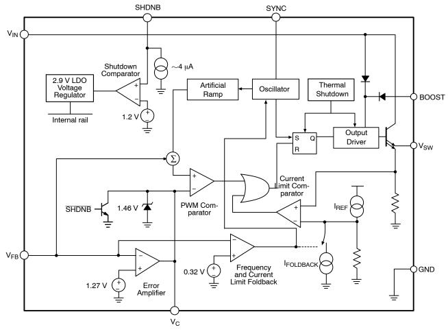
Figure 2. Block Diagram
