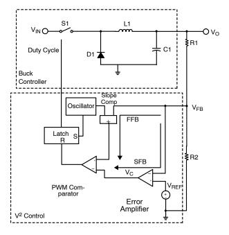
Figure 3. Buck Converter with V<sup>2</sup> Control.
