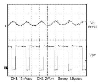
Figure 15. Output Voltage Ripple Using Two 10  $\mu$ F Ceramic Capacitors in Parallel
