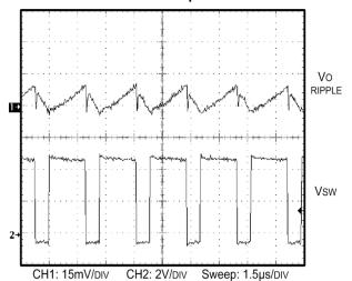
Figure 18. Output Voltage Ripple Using One 100  $\mu\text{F}$  Tantalum Capacitor
