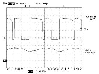
Figure 8. The Regulator in Current Limit
