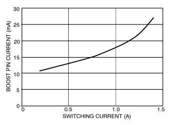
Figure 9. The Boost Pin Current Includes 7.0 mA
