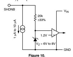
The IC enters a sleep mode when the SHDNB pin is pulled below the Shutdown Threshold Voltage. In sleep mode, the power switch is kept open and the supply current reduces to Shutdown Quiescent Current (1  $\mu A$  typically). This pin has an internal pull–down current. When not in use, pull this pin up to  $V_{CC}$  with a resistor (See Figure 1). A 100 k $\Omega$  pullup resistor will ensure safe operation from below 9 V and during a 40 V load dump condition.
