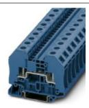
Feed-through terminal block with bolt connection, cross section: 0.1 - 2.5 mm², AWG: 26 - 14, width 12.3 mm, color: Gray
