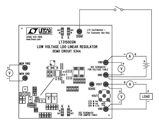
Figure 1. Proper Measurement Equipment Setup
