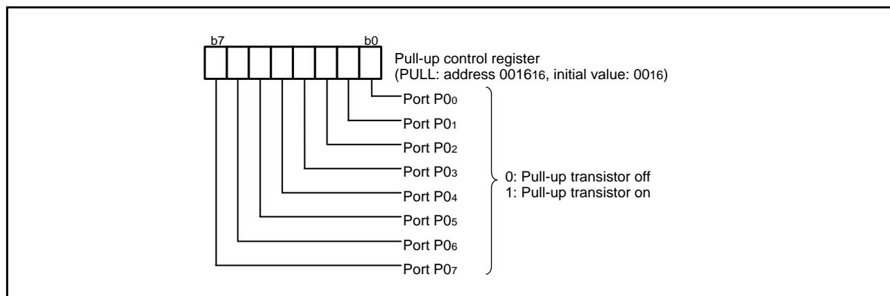
Fig. 13 Structure of pull-up control register
