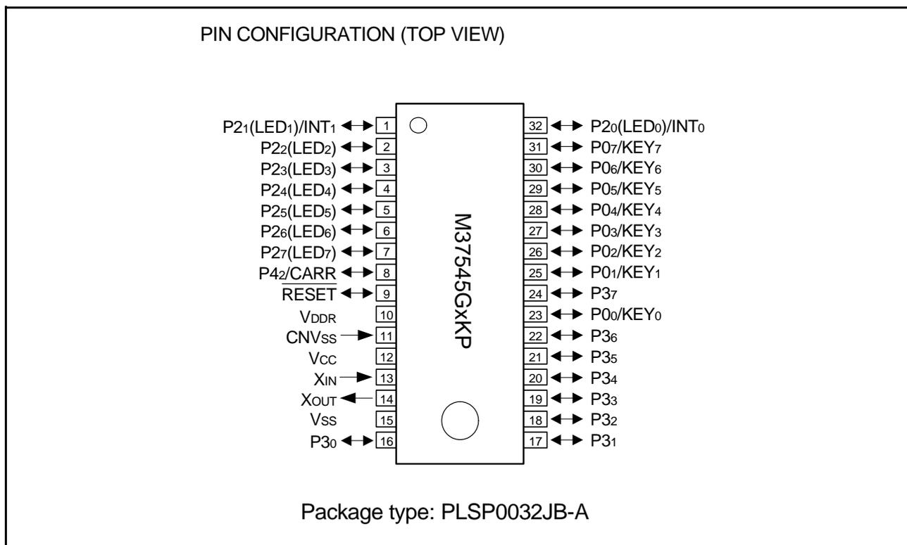
Fig. 2 Pin configuration (PLSP0032JB-A type)
