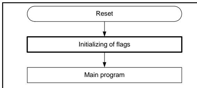
Fig 1. Initialization of processor status register
