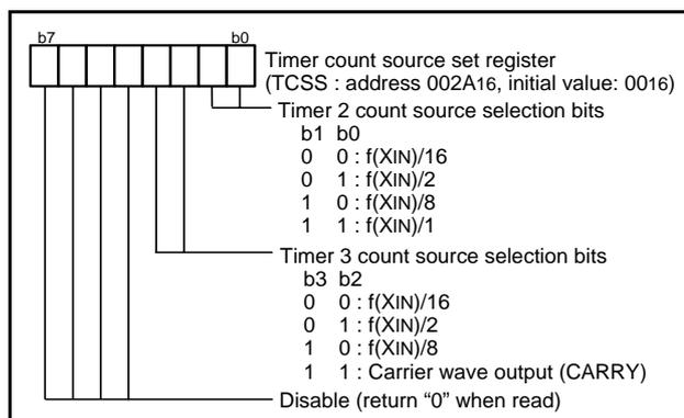
Fig. 22 Structure of timer count source set register
