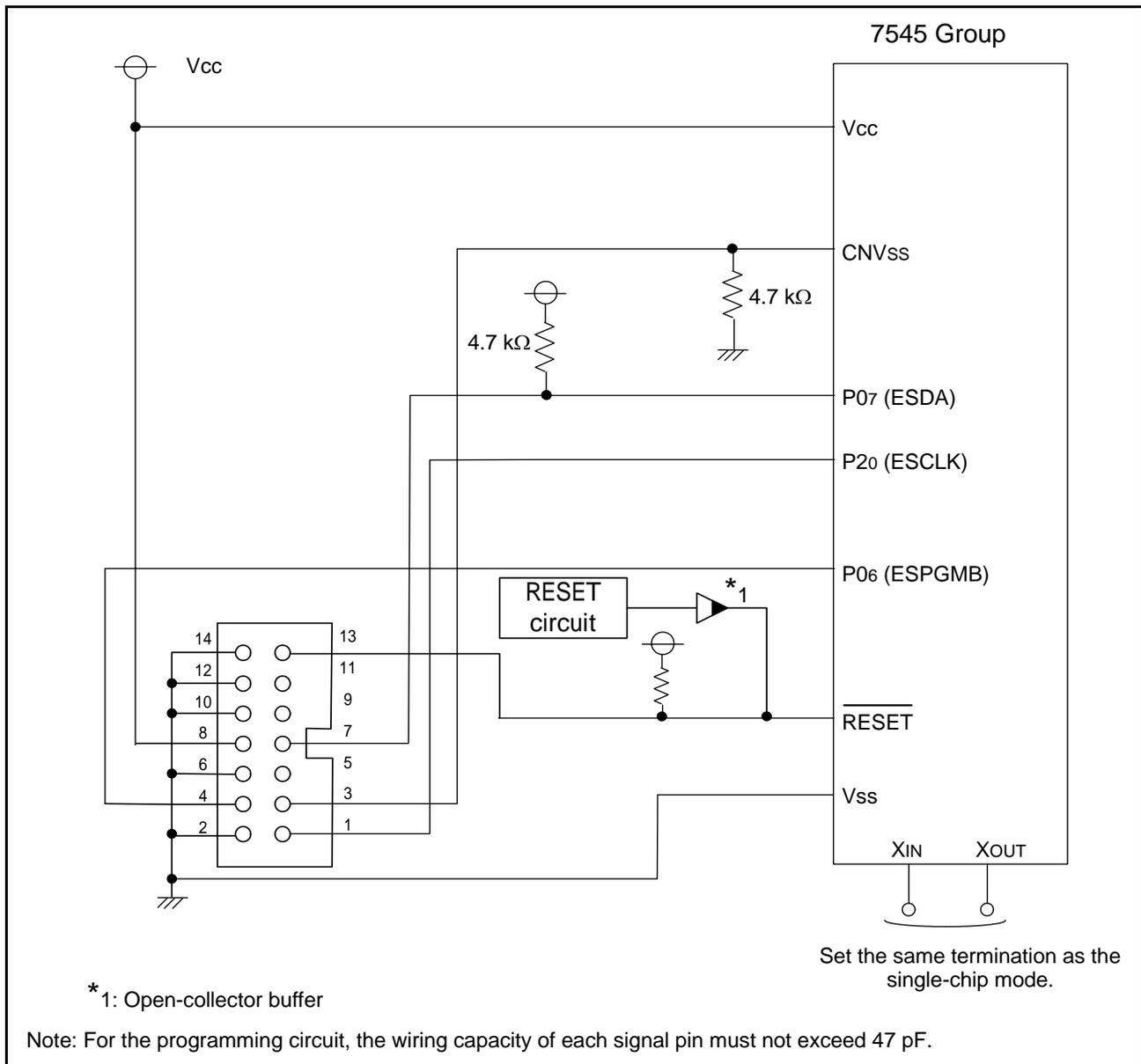
Fig. 46 When using E8 programmer, connection example
