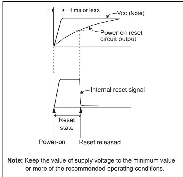
Fig. 36 Operation waveform diagram of power-on reset circuit
