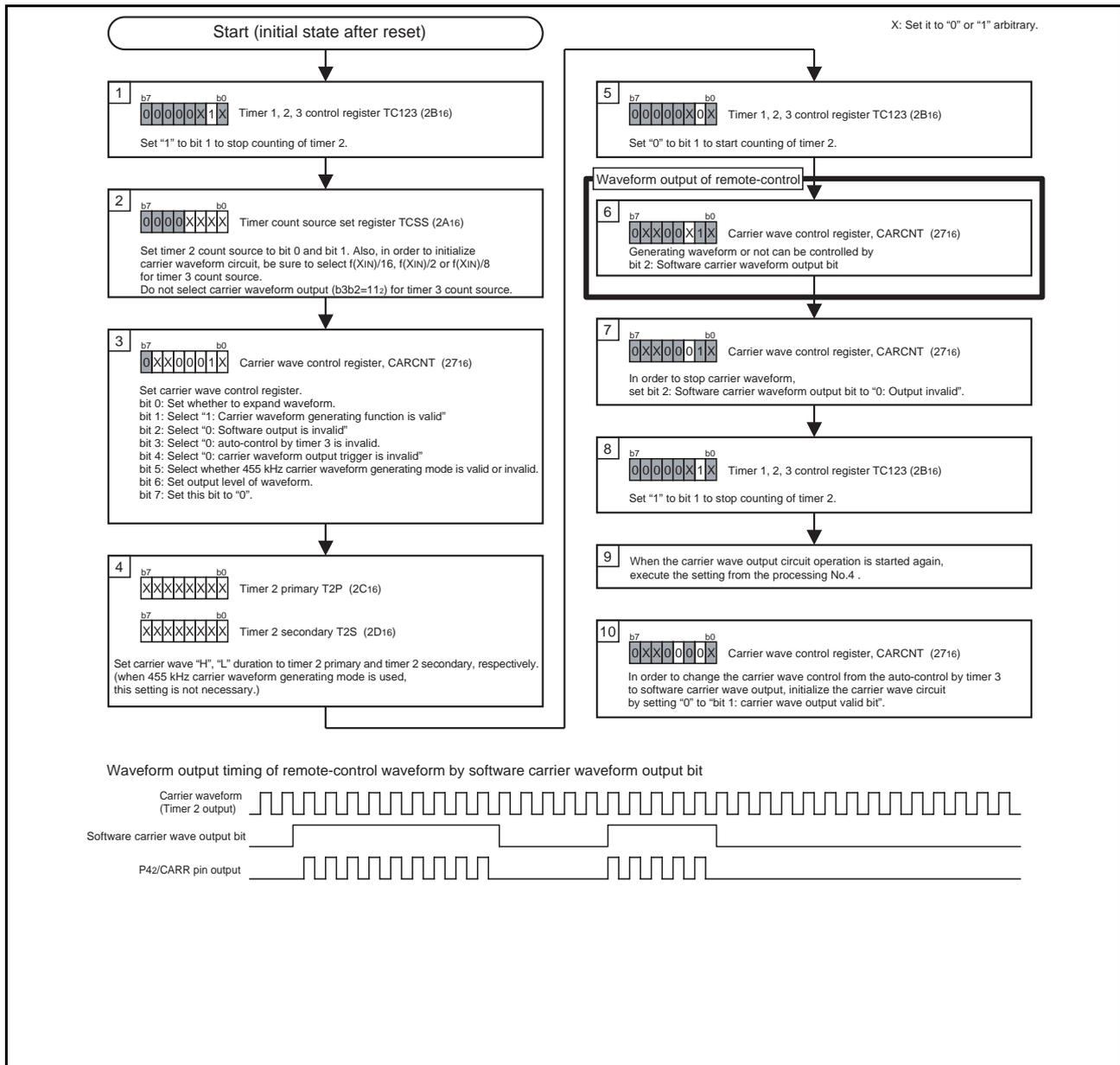
Fig. 32 Setting of carrier wave control by software
