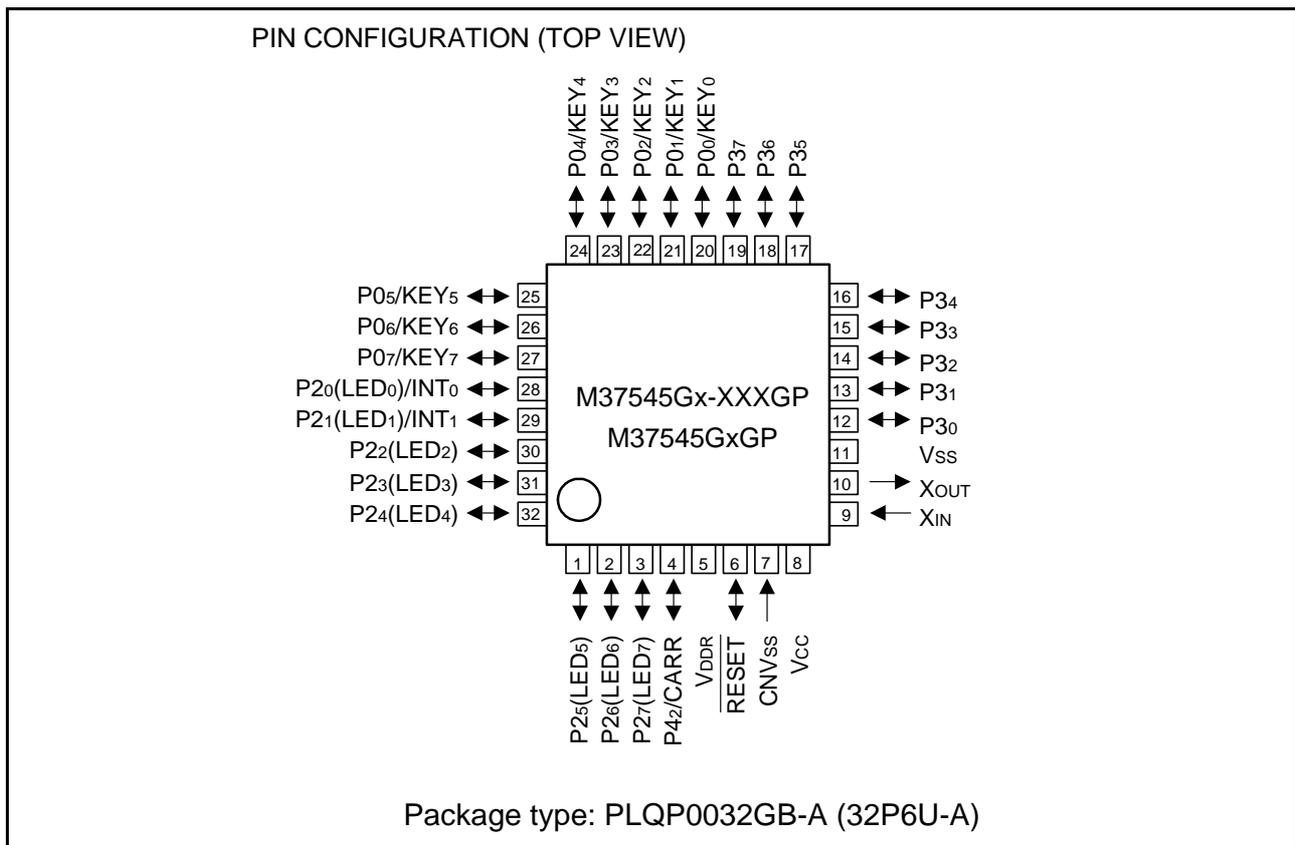
Fig. 1 Pin configuration (PLQP0032GB-A type)
