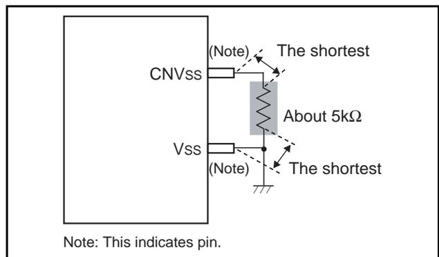
Fig. 51 Wiring for the VPP pin of the QzROM
