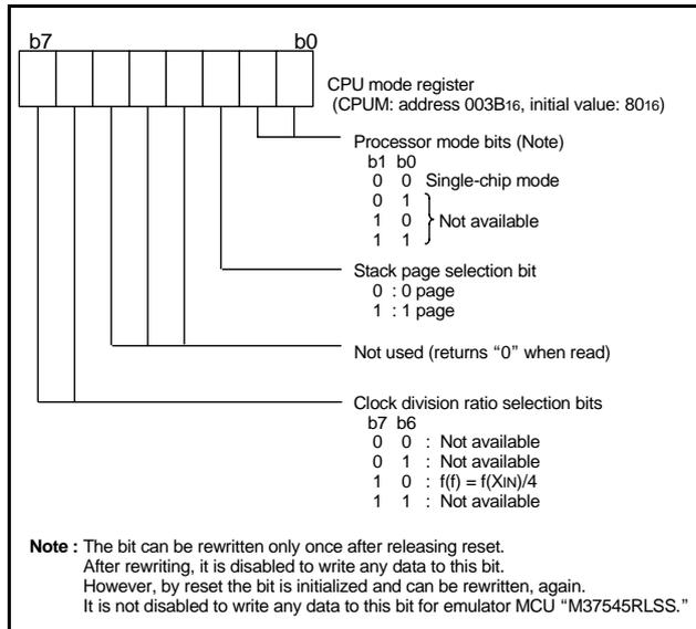
Fig. 9 Structure of CPU mode register
