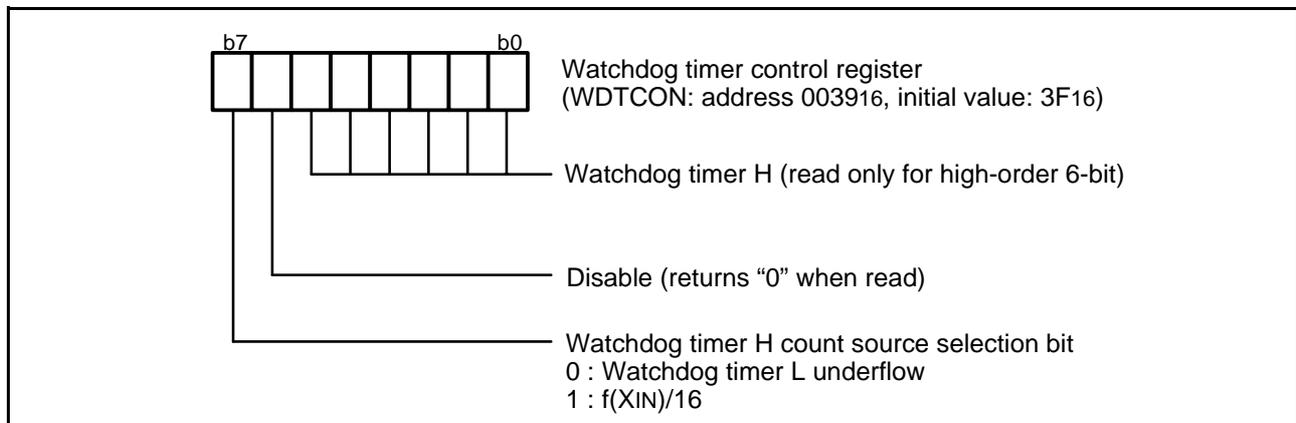
Fig. 33 Structure of watchdog timer control register
