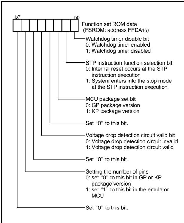
Fig. 12 Structure of Function set ROM area
