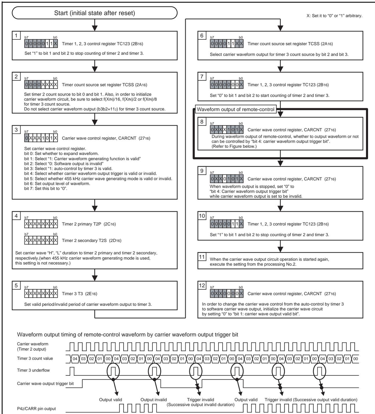
Fig. 31 Setting of carrier wave auto-control by timer 3
