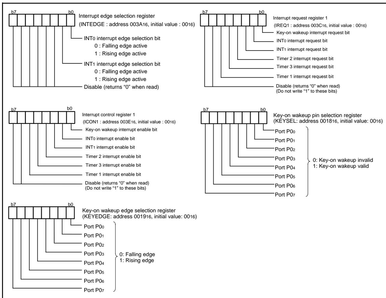
Fig. 17 Structure of interrupt-related registers
