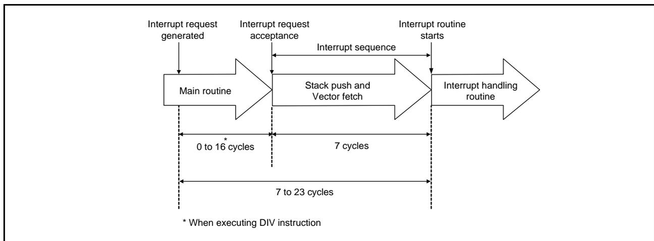
Fig. 18 Time up to execution in interrupt routine
