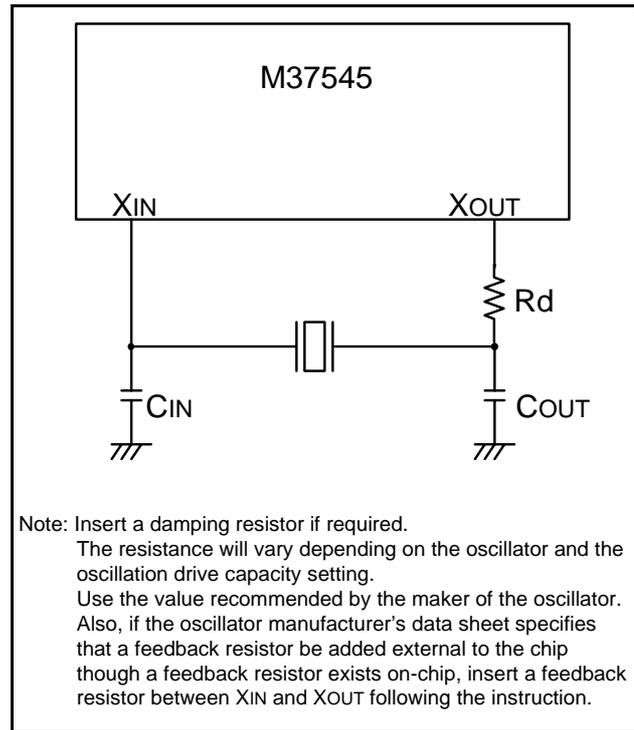
Fig. 41 External circuit of ceramic resonator/quartz-crystal oscillator
