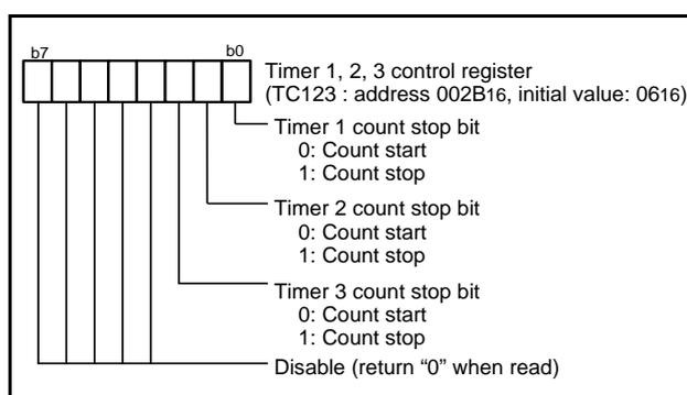
Fig. 23 Timer 1, 2, 3 control register
