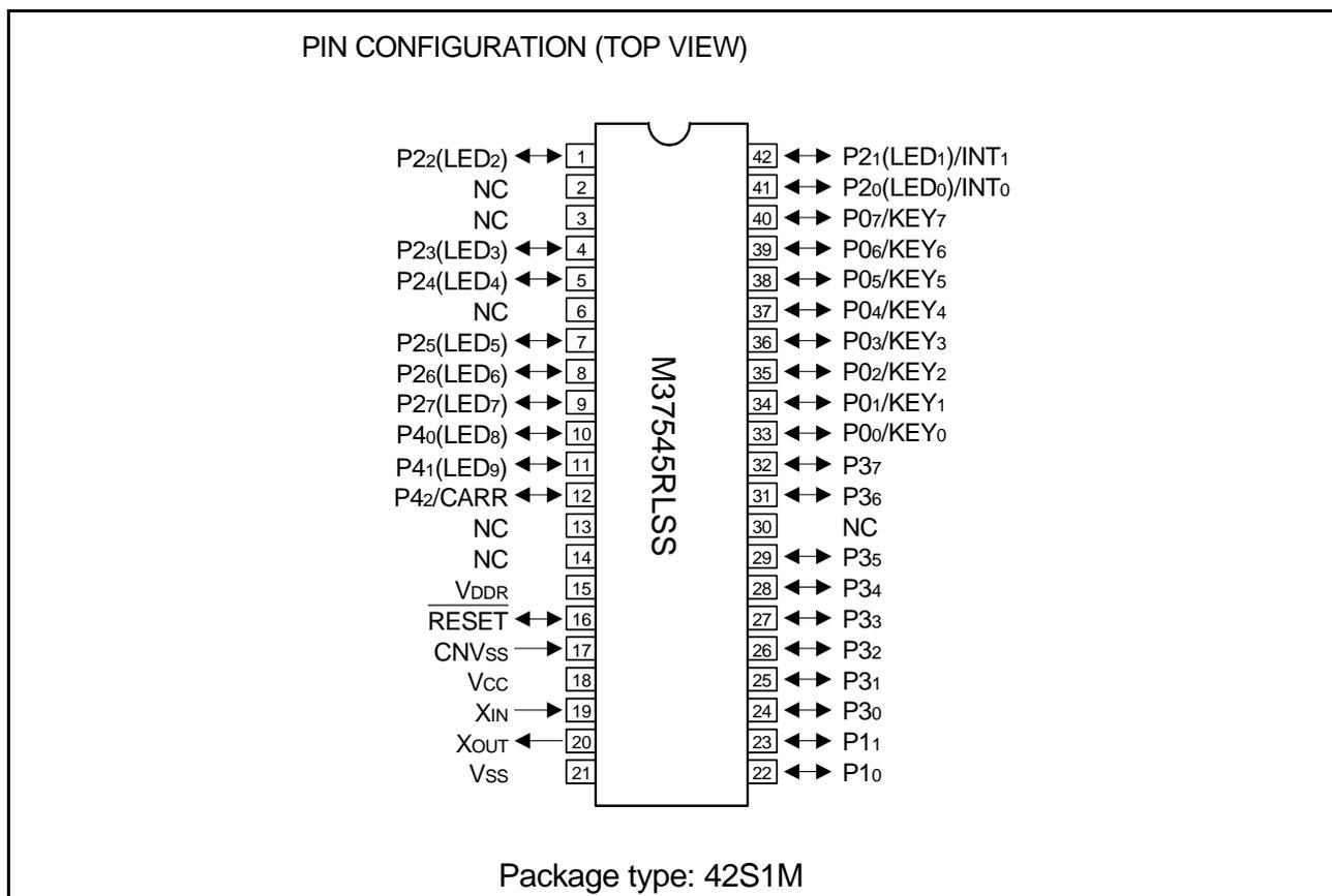
Fig. 3 Pin configuration (42S1M type)
