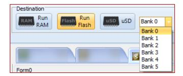
The additional drop-down menu allows the user to specify the target destination flash bank of the ViSi-Genie program. The Diablo16 processor has six flash banks (Bank 0 to Bank 5), each of which has a capacity of 32 kB.
