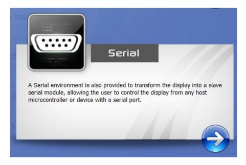
The **Serial** environment is provided to transform the module into a slave serial module, allowing communication and control from virtually any host micro-controller or device with a serial port.
