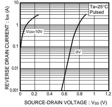
Fig.6 Reverse Drain Current vs. Source-Drain Voltage ( II )
