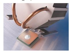
TIC™ 4000 is a thermally conductive grease compound designed for use as a thermal interface material between a computer processor and a copper-based heat sink. Other high watt density applications will benefit from the extremely low thermal impedance of TIC™ 4000.
