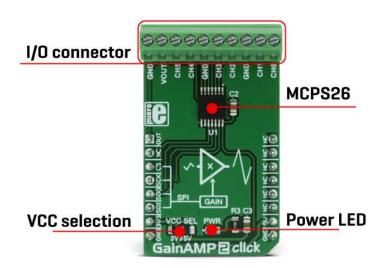
Besides the VOUT pin on the 10 pole I/O connector, the MCP6S21 output pin is also routed to the AN pin of the mikroBUS<sup>TM</sup> so it can be used as the input signal for the ADC. This allows the amplified signal to be easily digitalized and processed by the MCU. Using the click board in this configuration effectively turns the GainAMP 2 click into an analog port expander with the selectable gain on its inputs.
