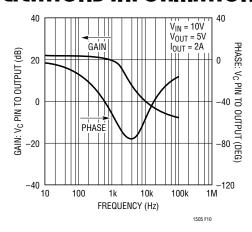
Figure 10. Response from V<sub>C</sub> Pin to Output
