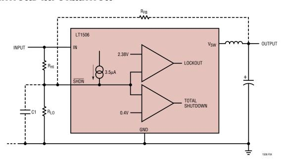
Figure 4. Undervoltage Lockout
