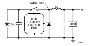
Figure 6. High Speed Switching Path
