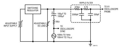
Figure 13. Loop Stability Test Circuit
