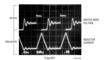
Figure 8. Discontinuous Mode Ringing
