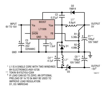
Figure 17. Dual Output SEPIC Converter
