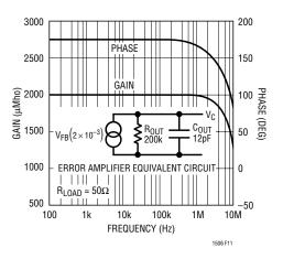
Figure 11. Error Amplifier Gain and Phase
