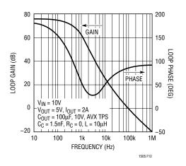
Figure 12. Overall Loop Characteristics
