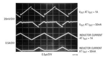
Figure 3. LT1506 Ripple Voltage Waveform
