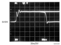
Figure 7. Switch Node Resonance
