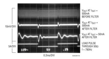
Figure 14. Loop Stability Check
