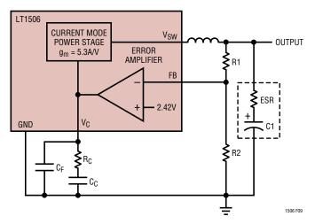
Figure 9. Model for Loop Response
