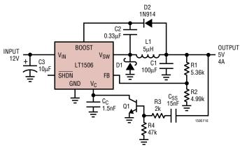
Figure 16. Buck Converter with Adjustable Soft Start
