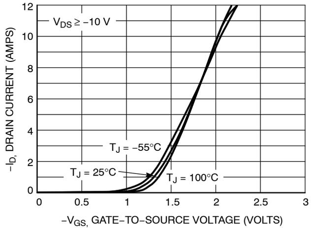
Figure 2. Transfer Characteristics
