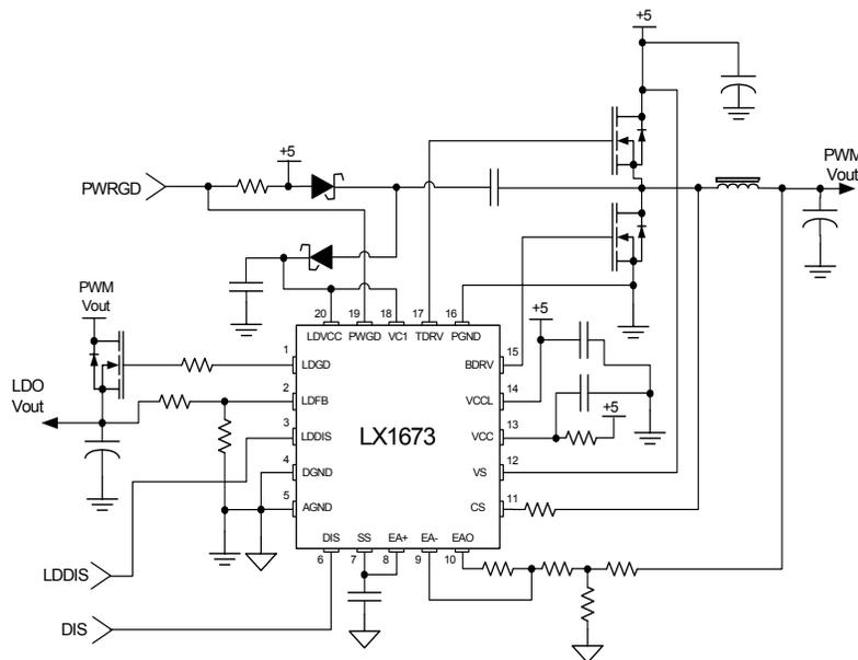
**Figure 4 – Schematic for 5 Volt only Input**
