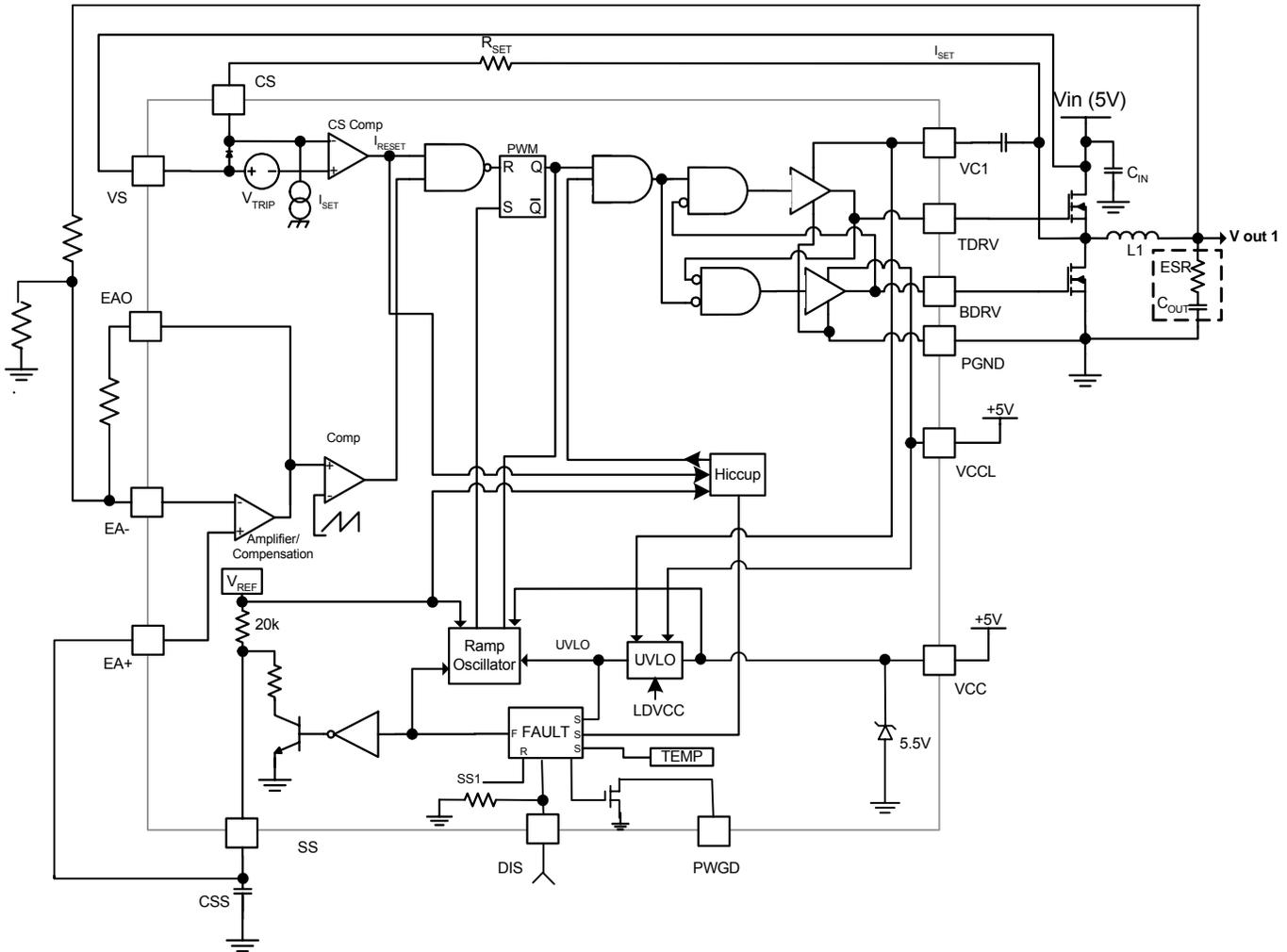
**Figure 1 – Block Diagram of PWM Phase**
