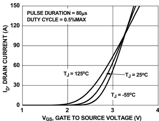
**Figure 5. Transfer Characteristics**
