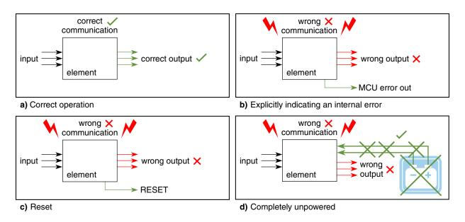
Figure 2-2. Safe state<sub>MCU</sub> of S32R274
