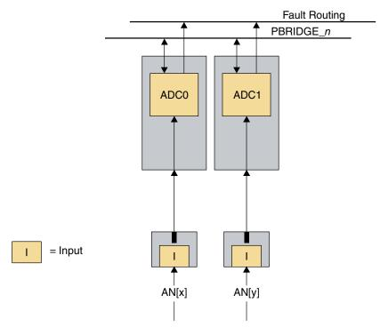
Figure 5-12. Double read analog inputs configuration
