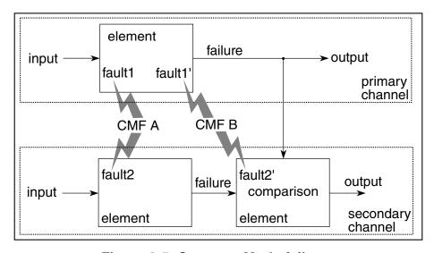
Figure 2-5. Common Mode failures
