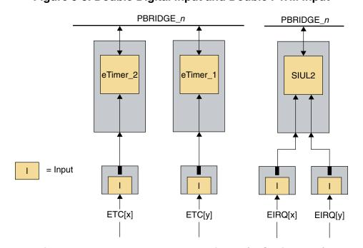
Figure 5-4. Double read encoder input (IRQ triggered)
