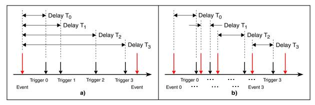
Figure 5-5. CTU operating modes: a) triggered and b) sequential
