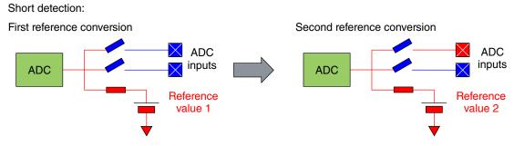
Figure 5-16. ADC\_SWTEST\_TEST2 (short detection)
