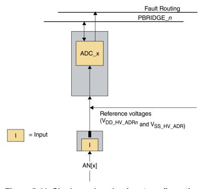
Figure 5-11. Single read analog input configuration
