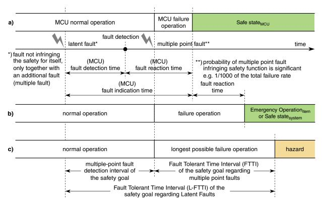
Figure 2-8. Fault Tolerant Time Interval for latent faults
