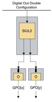
Figure 5-10. Double write digital output
