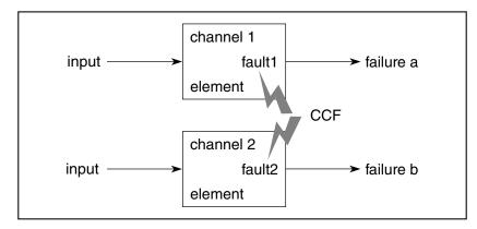
Figure 2-4. Common Cause Failures
