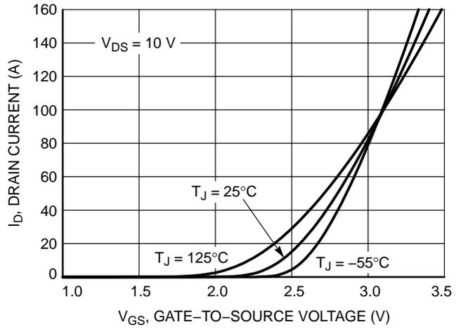
Figure 2. Transfer Characteristics
