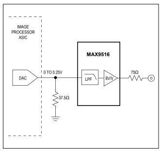
Figure 4. Video DAC Generates a  $0.25V_{P-P}$  Signal Across a  $37.5\Omega$  Resistor Connected to Ground
