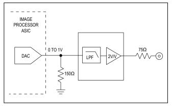
Figure 3. Video DAC generates a 1V<sub>P-P</sub> signal across a 150Ω resistor connected to ground.
