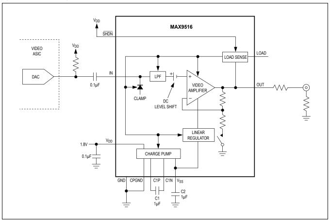
Figure 8. AC-Coupled Input
