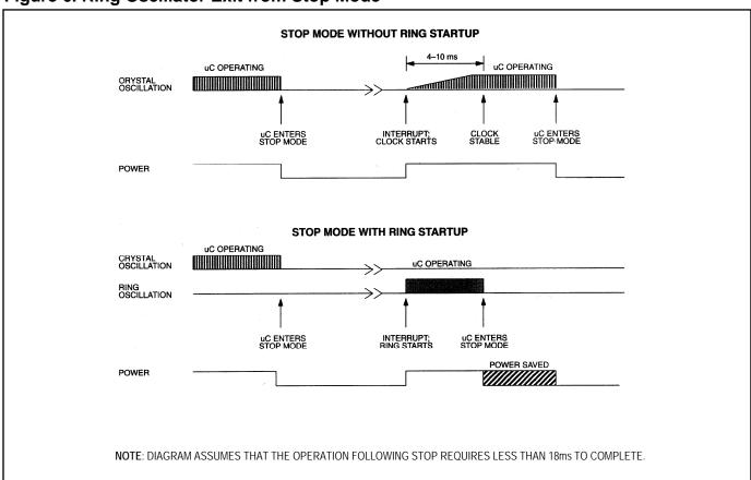
Figure 6. Ring Oscillator Exit from Stop Mode
