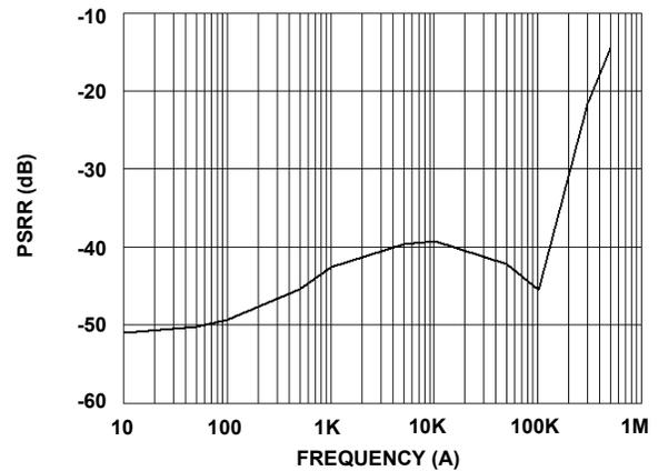
FIGURE 10. LDO1 POWER SUPPLY REJECTION
