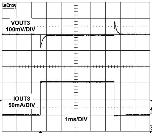
FIGURE 5. LDO3 LOAD TRANSIENT RESPONSE (10mA to 100mA)
