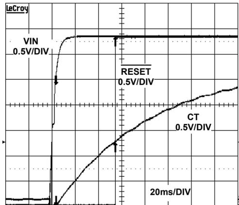
FIGURE 7. RESET DELAY DURING START-UP (CT = 0.01µF)
