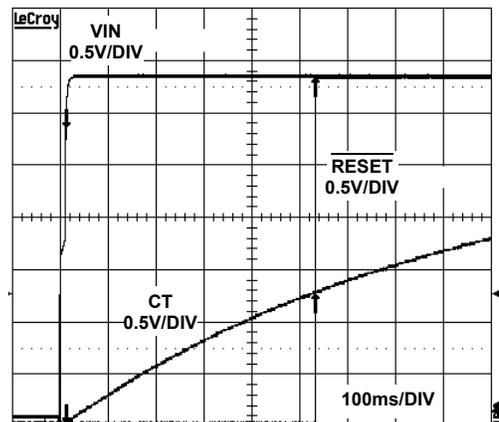
FIGURE 8. RESET DELAY DURING START-UP (CT = 0.1µF)
