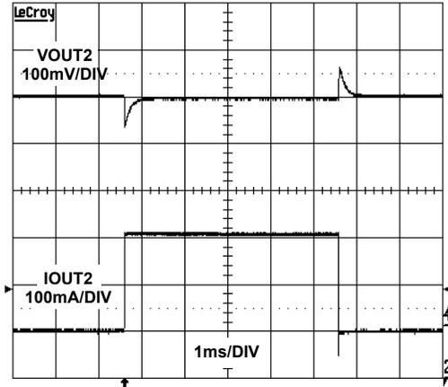
FIGURE 4. LDO2 LOAD TRANSIENT RESPONSE (10mA to 200mA)
