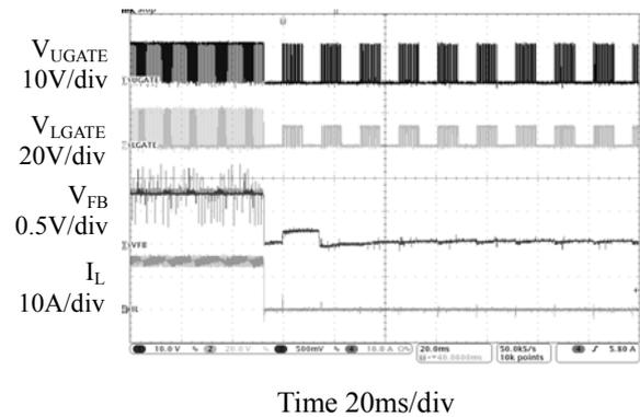
Figure 15. Under Voltage Protection
