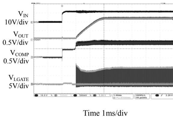
Figure 10. Power-on Waveform
