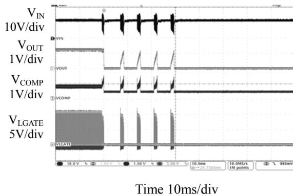
Figure 14. Over Current Protection
