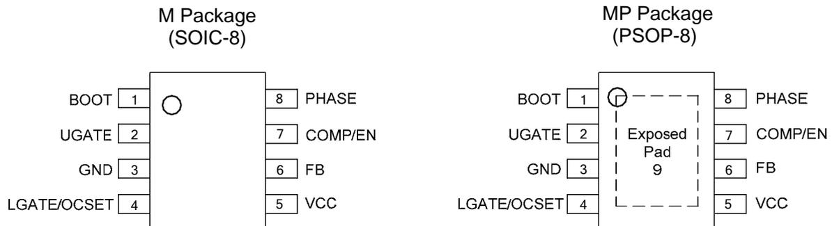
Figure 2. Pin Configuration of AP3586A/B/C (Top View)
