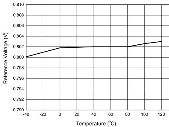
Figure 8. Reference Voltage vs. Temperature
