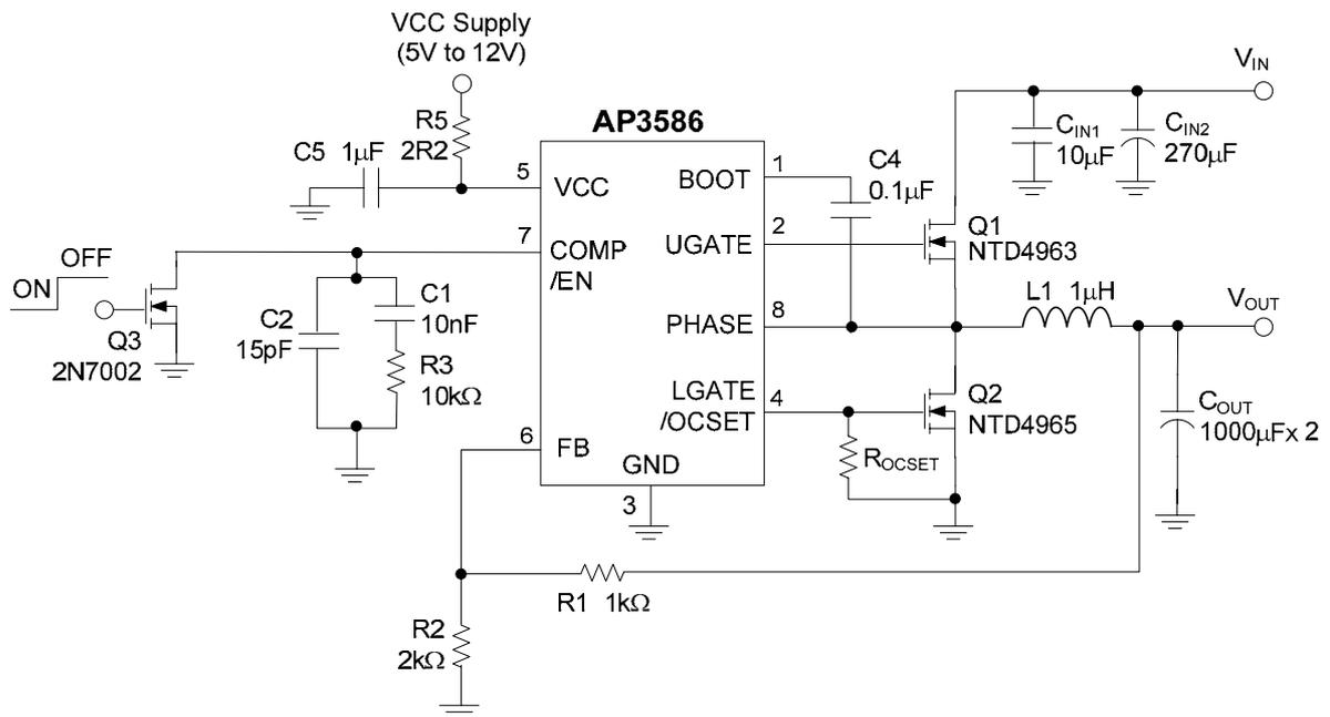
Figure 16. Typical Application Circuit of AP3586A/B/C
