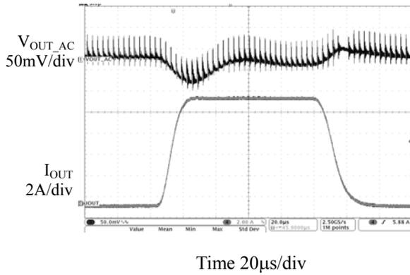
Figure 12. Load Transient Response
