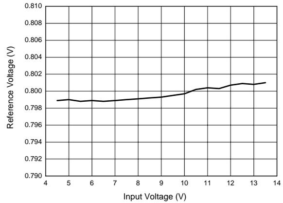
Figure 9. Reference Voltage vs. Input Voltage
