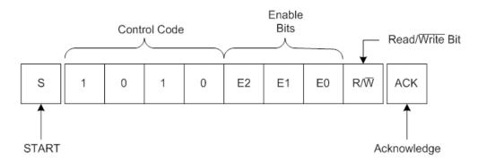
Figure 5-2. Control Byte, OTP Security Register Access
