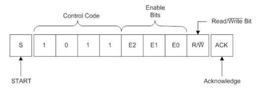
Upon receiving the correct Control Code, the chip enable bits, and the  $R/\overline{W}$  bit, the device performs an acknowledge by pulling the SDA line low during the 9th clock pulse. As stated above, the device will now be set for either a read or a write operation by the  $R/\overline{W}$  bit.
