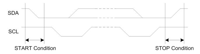
Every byte put on the SDA line must be 8 bits long. The number of bytes that can be transmitted per transfer is unrestricted. Each byte must be followed by an acknowledge bit; therefore, the number of clock cycles to transfer one byte is nine. Data is transferred with the most significant bit (MSB) first.
