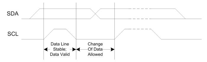
A high-to-low transition on the SDA line while SCL is high indicates a START condition. A low-to-high transition on the SDA line while SCL is high defines a STOP condition.
